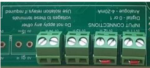
2. If the input is not used and a terminal bridge is installed (as shown in the diagram), ensure the input has been isolated in the software.
