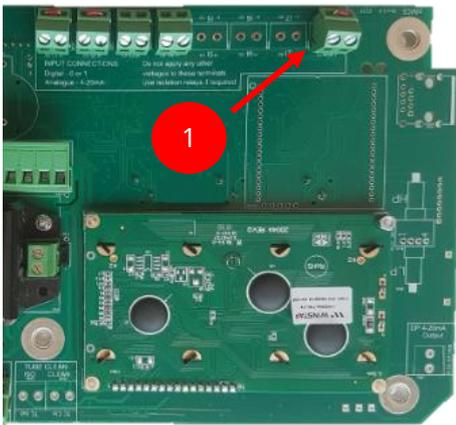
Connect the cables from input 8 (terminal J202 Clean) to the contactor on the normally open N/O motor controller.
