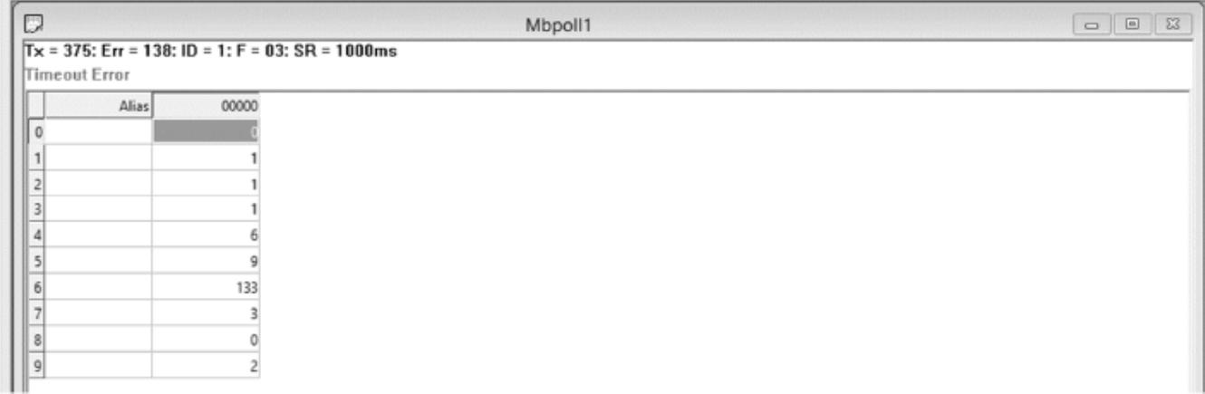
The screenshot shows a window titled "Mbpoll1" with a status bar at the top displaying "Tx = 375: Err = 138: ID = 1: F = 03: SR = 1000ms". Below the status bar, the text "Timeout Error" is visible. A table with two columns, "Alias" and "Value", is shown. The table contains the following data:
