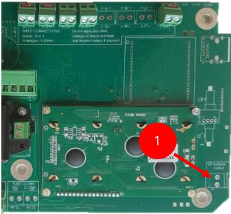
Connect the 4-20mA from the output terminal to the current loop isolation device. Do not connect the 4-20mA output directly to an external system.
