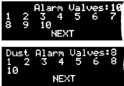
If the Controller has detected an electrical valve fault (short or open circuit) or broken bag, then a matrix of faults will be displayed. This assists the user to identify where the fault has occurred.
