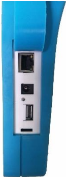
Power, USB Disk, RJ45 port
