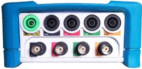
Current and voltage input
